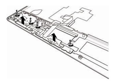
Figure 4-22 Removing the LED and Fingerprint Board
